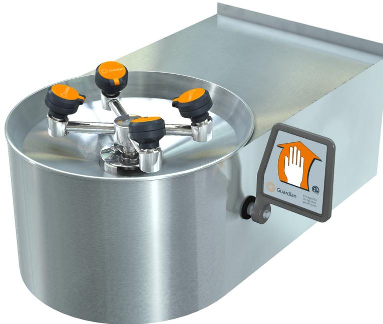
**APPLICATION:** Handicapped accessible WideArea™ eye/face wash for wall mounting. Bowl is lowered and extended to permit access by wheelchair user. Profile of unit is “flattened” to comply with maximum height and knee clearance requirements. Unit has stainless steel bowl and wrap around skirt to conceal valve, drain and piping.
