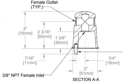
Drill Ø1/4" Mounting Hole in Counter Surface for Vandal Resistant Pin
