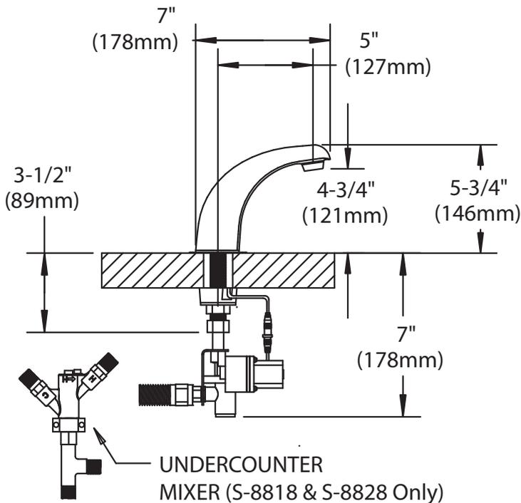
NOTE: Position faucet as close to the edge of the sink as possible. Ensure adequate clearance for wire protector, wires, washers and nut. Unless otherwise specified, all inlets are 3/8 compression with male threads. Unless otherwise specified, all dimensions are in inches and are subject to change without notice.
