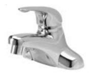
Engineering Specifications: Zurn AquaSpec® Sierra Lead-Free Faucet Z7440 Polished chrome plated 4"[102mm] centerset single control lavatory faucet with 5" [127mm] integral spout, a ceramic disc cartridge and a temperature limit stop. Unit is furnished with 2.2 GPM [8.3L] aerator (complying with ANSI A112.18.1M Standard for flow), an ADA compliant lever handle, 3/8" stainless steel flex hose 18" [457mm] in length with 3/8" female compression fitting.
