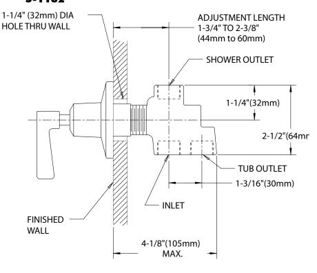
NOTE: All dimensions are in inches (millimeters) unless otherwise specified and are subject to change without notice. Inlet and outlets are 1/2" NPT female.
