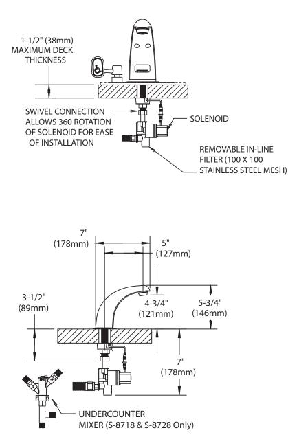
NOTE: Position faucet as close to the edge of the sink as possible. Ensure adequate clearance for wire protector, wires, washers and nut. Unless otherwise specified, all inlets are 3/8 compression with male threads. Unless otherwise specified, all dimensions are in inches and are subject to 184 change without notice.
