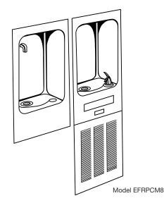
**Cuspidor Body:** One piece #18 gauge stainless steel, type 304. Anti-splash design. Extends only 1/2" from finished wall after installation.
